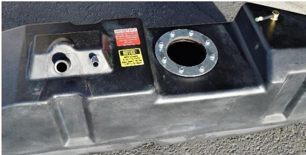
(Fig. 10) Install the OEM 1 ½" fuel tank fill hose to the large king nipple and the ¾" OEM vent hose to the smaller nipple. Be sure to fasten tightly with the OEM hose clamps.
