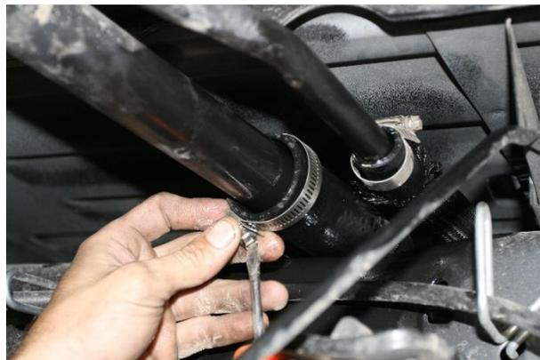
(Fig. 11) Attach fuel tank 1 ½" fill hose and ¾" vent hose to vehicle fill spout. On some long-bed tanks, 1 ½" fill hose may have to be extended with 3.25" hose extension.
